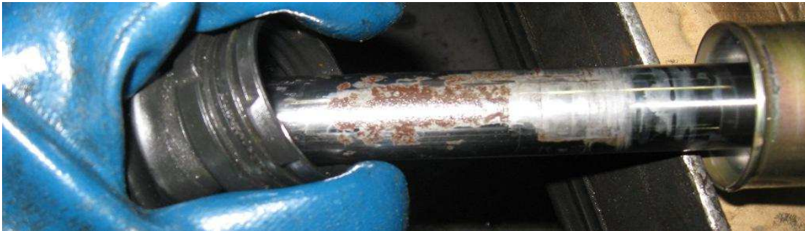
NOT GOOD - Rusty rack
