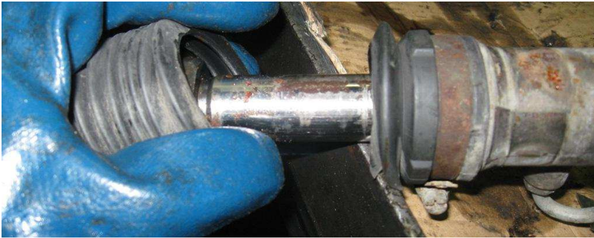
NOT GOOD - Rusty rack
