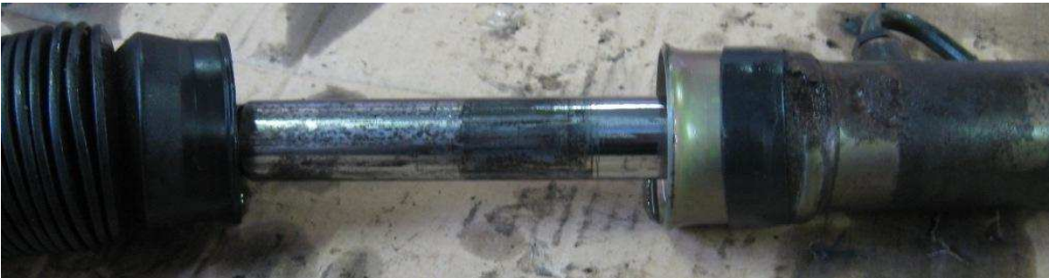
NOT GOOD - Rusty rack
